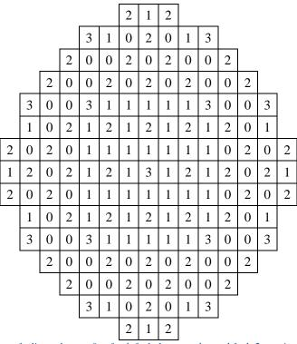
Figure 12. A low-leakage core refueling scheme: 0 = fresh fuel; 1 = once burned fuel; 2 = twice burned fuel; 3 = third burned fuel [8].
