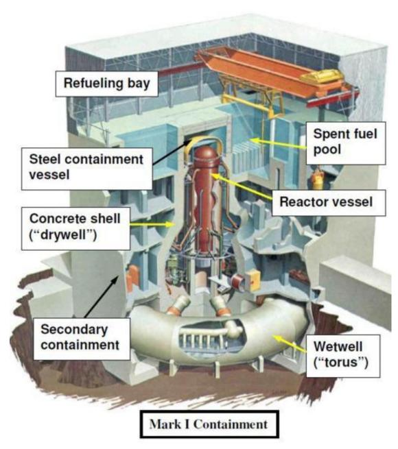
Figure 26. Illustration of the BWR containment building systems.
