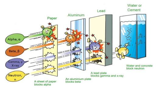
Figure 2. Illustration of stopping power for different types of radiation.
