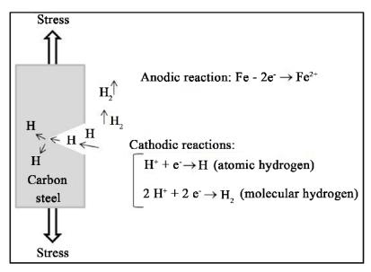
Figure 32. Illustration of stress corrosion cracking process.
