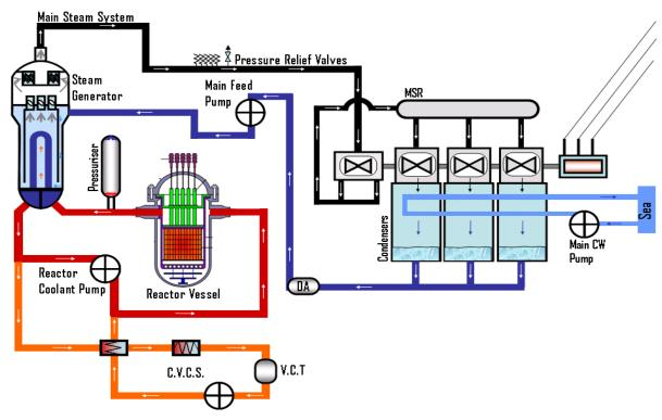
Figure 19. Diagram of the PWR system layout.
