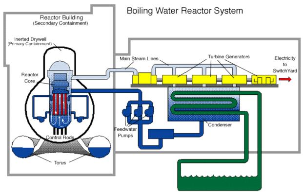
Figure 25. Diagram of the BWR system layout.
