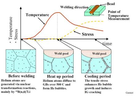
Figure 38. Mechanisms of He induced weld cracking.
