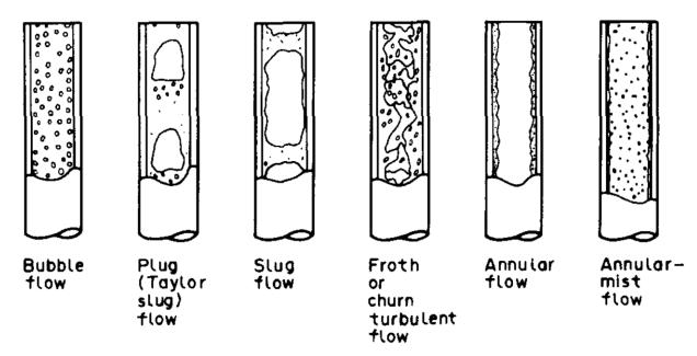
Figure 17. Schematic of the different flow regime in a vertical pipe [9].
