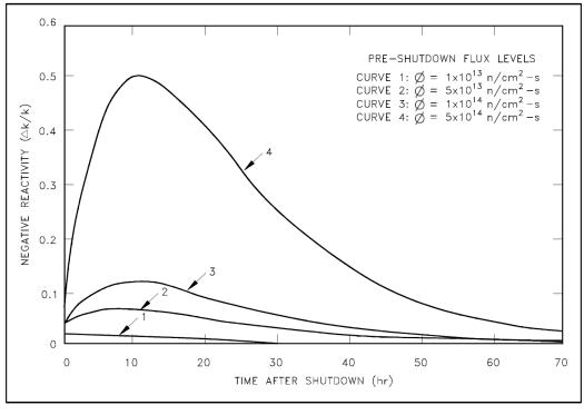
Figure 10. Xe-135 reactivity after shut-down [7].
