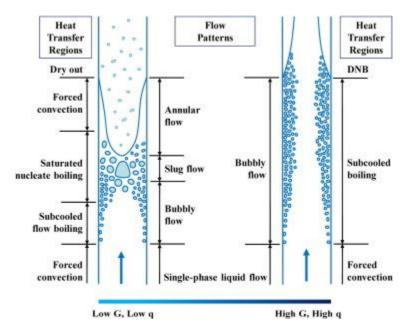
Figure 18. Schematic of two different types of CHF mechanisms. G refers to the mass flux, and q to the heat flux here [10].
