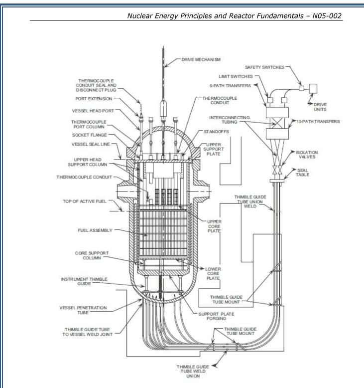
Figure 42. PWR In-Core Instrumentation [23]
