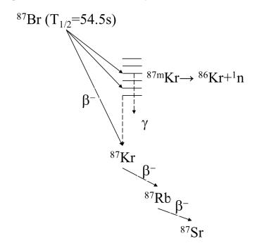
Figure 11. Production of a delayed neutron from the Br-87 decay chain.
