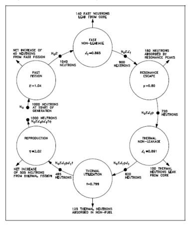
Figure 7. The neutron life-cycle for thermal reactors [7].
