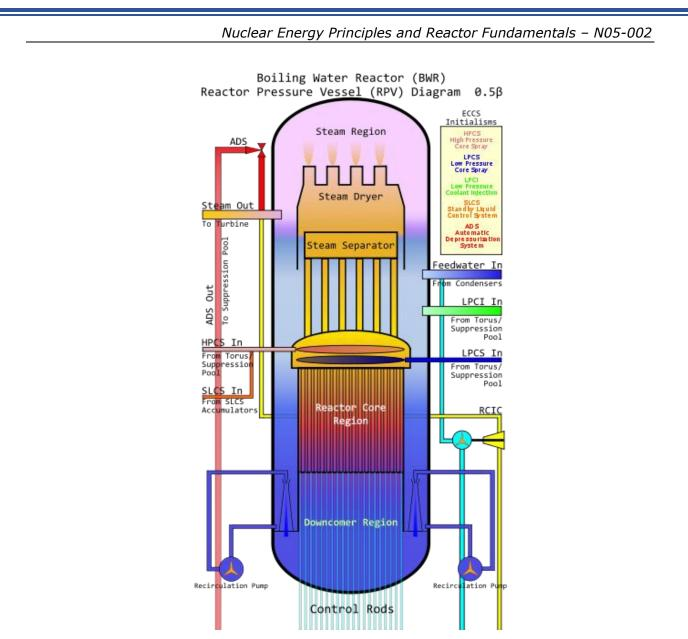
Figure 27. Cross-section view of the BWR pressure vessel.
