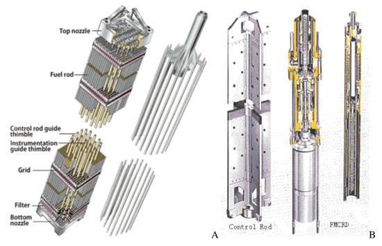
Figure 13. PWR fuel assembly with control rod "spider" clusterr (A), BWR control blade (B).
