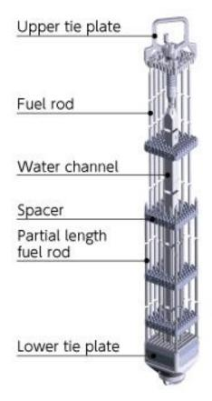
Figure 28. Layout of the BWR fuel assembly.
