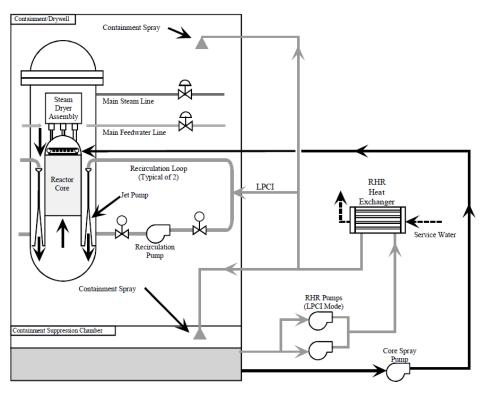
Figure 30. Diagram of the BWR low pressure Emergency Core Cooling System [13].
