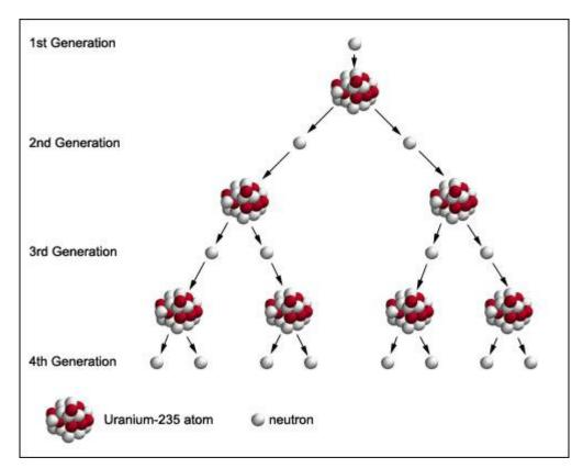
Figure 6. Illustration of the neutron chain reaction [6]
