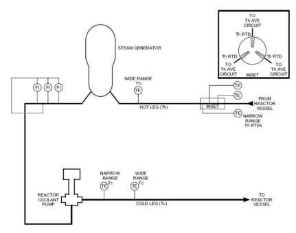
Figure 40. Simplified sketch of the PWR RCS loop instrumentation without bypass manifolds. T<sub>h</sub> stands for hot leg temperature. Tc stands for cold leg temperature [21].
