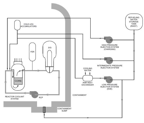
Figure 24. Diagram of the PWR Emergency Core Cooling System [12].
