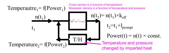
Figure 9. Illustration of neutron feedback with thermal-hydraulic influences.
