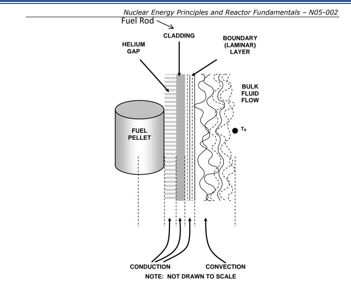
Figure 15. Overview of the heat transfer through a reactor fuel rod and into the coolant.
